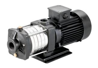
C.R.I. Horizontal Multistage centrifugal pumps are powered by a Totally Enclosed Fan Cooled, A.C. induction motor, suitable for continuous duty. Motor stator is made of low watt loss steel laminations assembled under pressure and rigidly locked in the frame. Dynamically balanced rotor ensures vibration and noise free operation and the varnished impregnated windings made of enameled copper wire offer excellent resistance.
